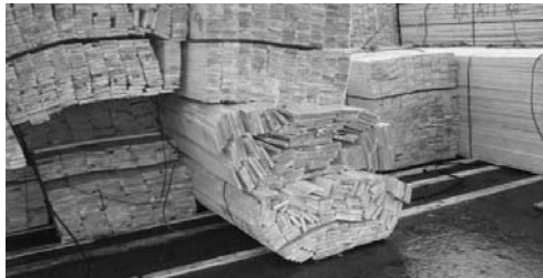
Figure 6.2. Example of poor rigidity
