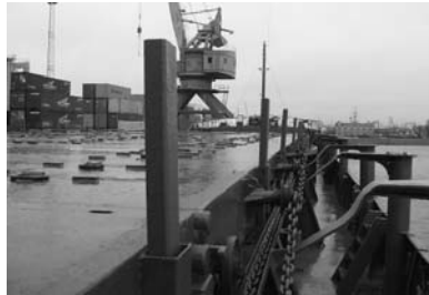
Figure 6.7. Example of uprights for bottom blocking
